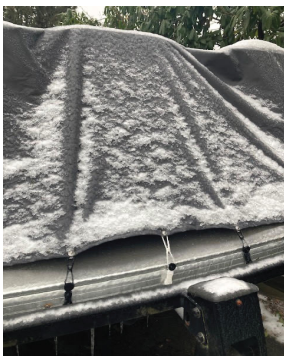
STREX fasteners holding strong in freezing temperatures after pontoon boat cover filled with 30 gallons of water and ice.
